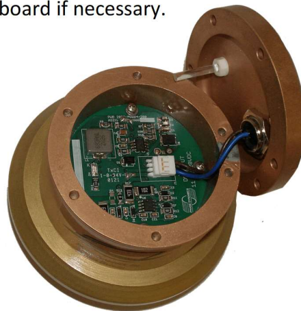
3" Configuration, DC Circuit Board with Lid, Connector & Light Pipe
